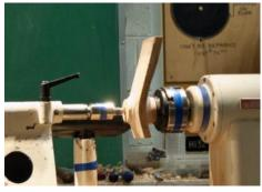
Once the proper depth has been achieved for the bowl it can be sanded in the inside—carefully! Using a jam chuck in the jaws, he then shapes the base to conform to the top curve and removes the tenon.
