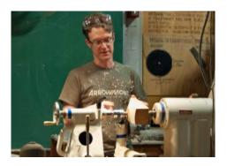
Mark uses a 1/2 inch bowl gouge and a pulling cut to form the underside shape. Pulling and using 1/3 of the wing makes interrupted cuts easy.
