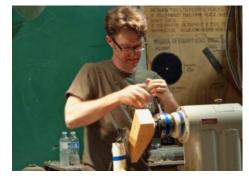
The piece is reversed and put in a 4jaw chuck. The tenon is carefully made with a slight dovetail shape so as to pull the piece into the jaws.
