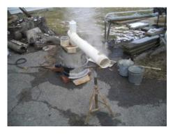
On March 23, I fired up my steam box again. This is a jury-rigged device with a propane weed burner boiling water in a rescued aluminum dye pot. A lid was turned from a failed bowl blank with a rabbit to fit the pot-rim on one side a 1 ½" hole in the center and a flange for forcing on 3" PVC Sch. 40 sanitary drain pipe. This rig delivers 212 degree F steam to the end of a 4-foot steam chamber. I steamed and bent
