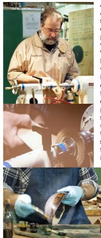
After stepping away from the poster board, Andy got into the hands on part of the demonstration. He began by showing us how you could simulate sandblasting without the expense of a sandblaster. Simply mount a brass wire wheel on your lathe and abrade that bowl. Want something more low tech, buy a wore brush! Andy then turned to dying different woods, with the admonition that you should try it on scrap wood first. After sanding back a dark colored dye, he showed the dramatic ef-
